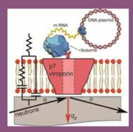
The cell-free preparation of supported bilayers containing p7 and NR and EIS measurements (not to scale). For neutron reflectivity, membranes were formed on quartz and an incident neutron beam was transmitted through the substrate and reflected from.
